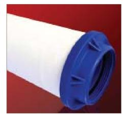
Parker domnick hunter's solvent & caustic coalescer with high performance nylon 66 media is designed to remove carried-over water and caustics from hydrocarbons. Common materials of construction used in coalescing elements are often not compatible with aromatics. The proprietary nylon 66 coalescing media is designed specifically for aromatics and caustics.
